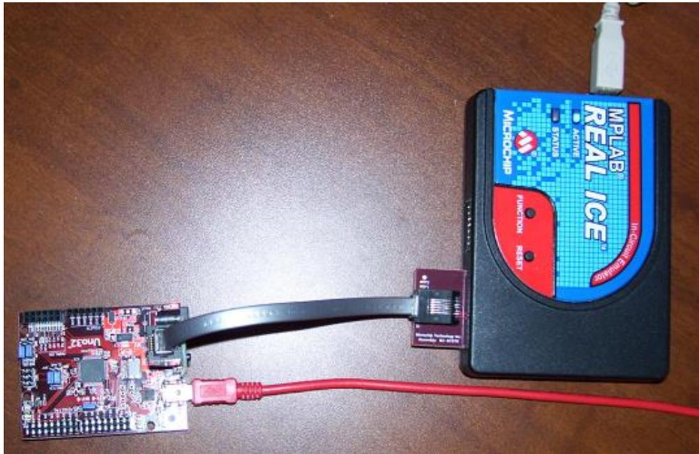
In the image below, you can see the RJ-11 socket to ICSP adapter. The RJ-11 cable can be coming from either the MPLAB REAL ICE or the MPLAB ICD 3.
